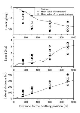
Figure 1 Ship-handling results of the 3rd grade trainee
